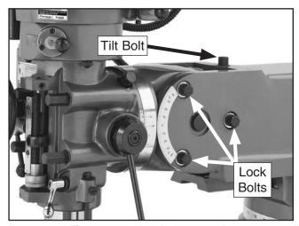
Figure 22. Head tilt controls.
